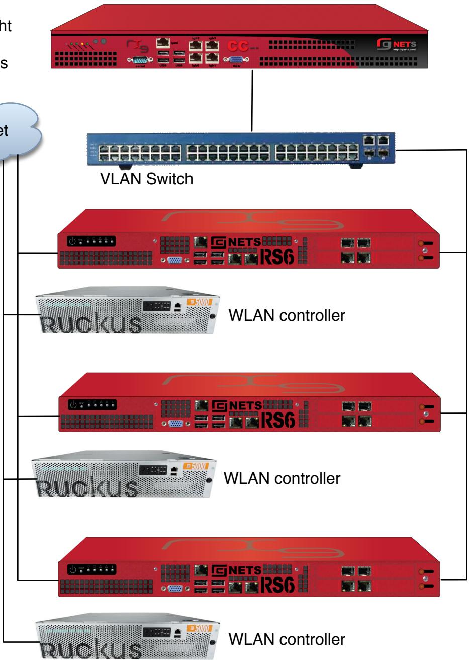
Centralized rXg RS6 cluster nodes deployed side by side with WLAN controllers that are the endpoints for tunnels originating from geographically distributed APs.
